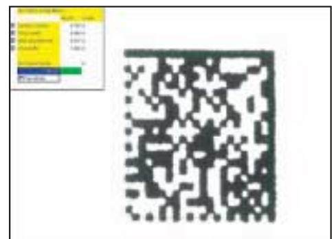
ISO 16022 metrics are recommended for codes made up of square cells with continuous L pattern.
